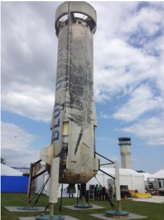
Left: Blue Origin rocket has been into space five times. It returns for a vertical landing. Called the New Shepherd after Allen Shepherd who
