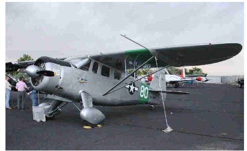
1944 Howard DGA-15P w/ Pratt & Whitney R-985 radial engine, N115P is painted in WWII Navy colors. Owned by Brian Longwill of Albuquerque.
