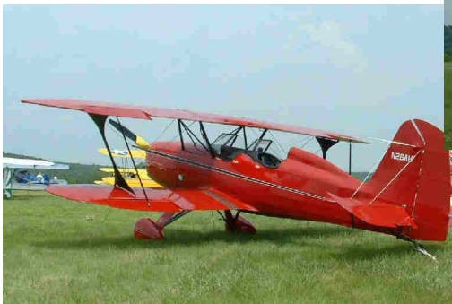
Above— Starduster II powered by an inline Fairchild 6-440 engine.
