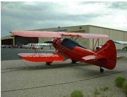
Left- 1940 Waco UPF-7 w/ Continental W670 radial engine, NC32016 owned by Gregory Sullivan of Albuquerque.
