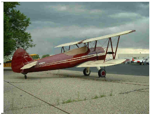
Right- 1941 Boeing Stearman E75 w/ Pratt & Whitney R-985 radial engine, NC4787V owned by Golden Wings Advertising, Inc of Albuquerque.
