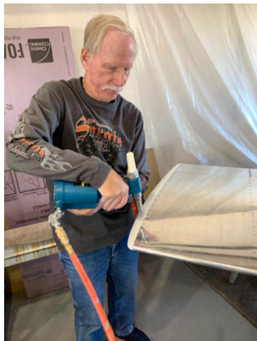
Mark Dyslin riveting the fiberglass caps on the rudder, vertical stabilizer and horizontal stabilator.
