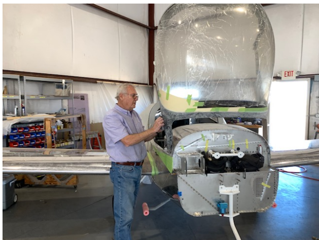
Lee Otto fitting, sanding, and filling the fiberglass windscreen fairing.
