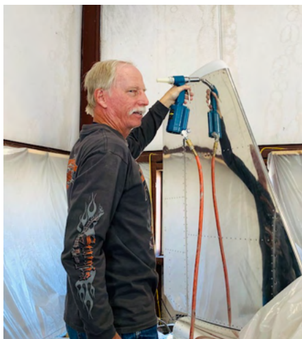
Mark Dyslin riveting the fiberglass caps on the rudder, vertical stabilizer and horizontal stabilator.
