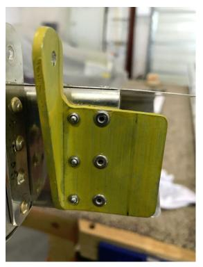
We've been working on the finishing the flaperons and sealing the firewall. As you might remember when we got the fuselage kit and the wings we only got one flaperon and we had to order skins and ribs to complete the second one. That has now been done and the last items we needed to finish were the two flaperon actuation brackets.
