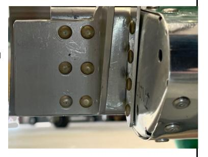
You can see in the pictures of the brackets how they were made and attached by the previous owner. We will also work on completing all the service bulletins not yet completed for the airplane so that it's up to date with the latest version of the plans.
