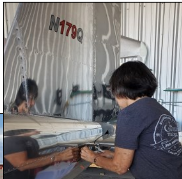
Attaching the official Aircraft ID plate.
